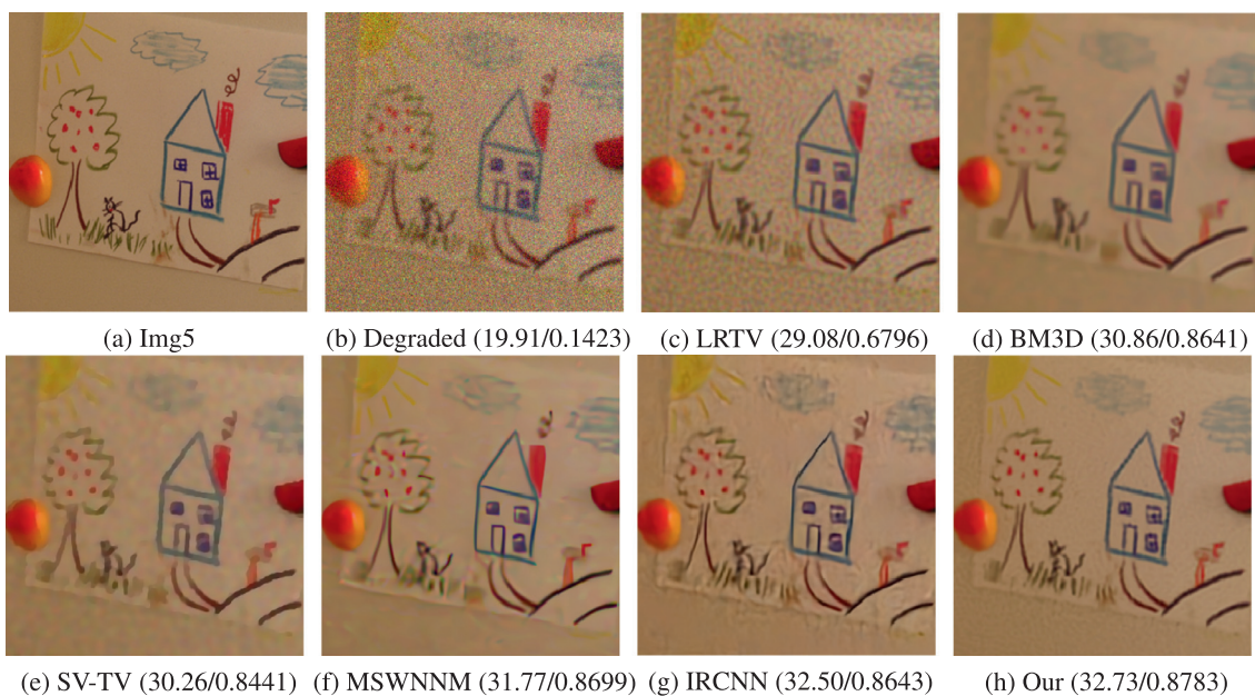
Fig. 7. Zoom in part of color image restoration on Img5 with visual quality and numerical results (PSNR/SSIM). (a) original image, (b) degraded image with Gaussian kernel (25, 1.6) and Gaussian noise level \sigma = 25 , restored image reconstructed by: (c) LRTV [37], (d) BM3D [40], (e) SV-TV [17], (f) MSWNNM [38], (g) IRCNN [35], (h) our QWNNM.
